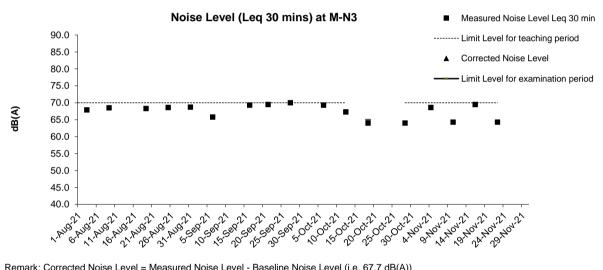
Remark: Corrected Noise Level = Measured Noise Level - Baseline Noise Level (i.e. 67.7 dB(A))
